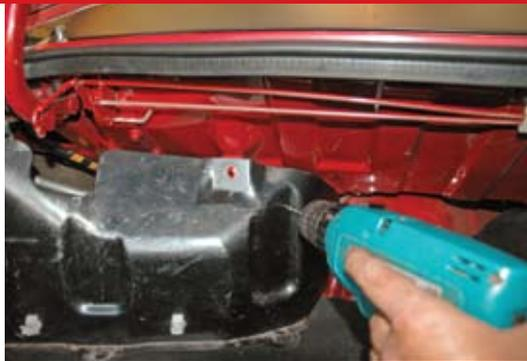
STEP 1: Drill the first hole and place a bolt through the mount to keep the mount in place while you drill the remaining holes.
