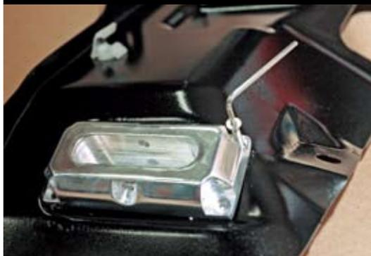
STEP 3: The flush-mount allen-head screws look great, and will hold up well if you use nuts on the backside of the bulkhead.
